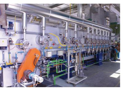
The new heat treatment line can be remotely controlled by a computer system enabling Mecavit to manage, recover and reuse the heat produced, contributing to energy savings.
